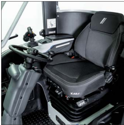
Decoupled driver's cabin with air-suspended comfort seat, seat heating and longitudinal damping
